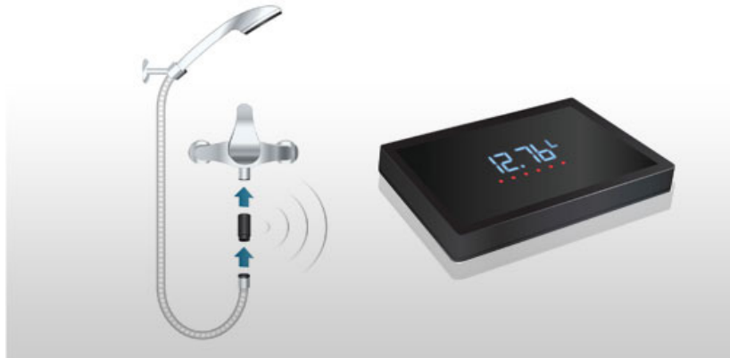
Figure 2. Installation of the Smart Water Meter (Amphiro AG)
