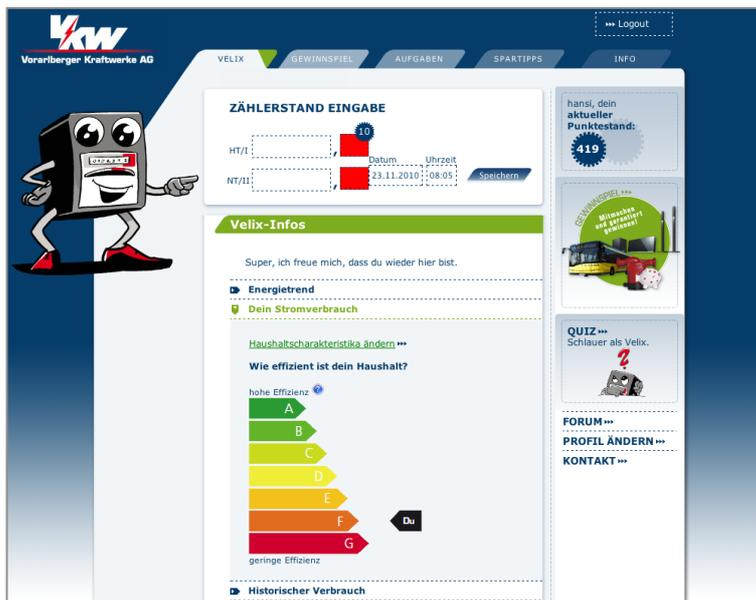
Figure 1. Screenshot of the persuasive web application Velix. Shown is the feedback page where users can enter their electricity meter readings and receive feedback on their energy efficiency.
